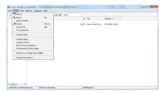
**FLASH2GUI's** Image Editor facilitates data backup and restore based on a bit-for-bit disk image which can be unpacked, edited, re-packed and restored direct the **SCSIFlash™** and **FLOPPYFlash™** drive. It also enables the creation of a new formatted drive and the addition of new software install files to run from the drive.
