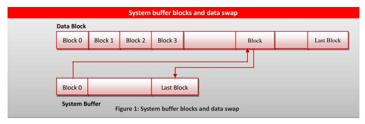
In the worst case scenario the host keeps writing data to Block N while the system buffer blocks are used frequently and the other data blocks are not used at all. All system buffer blocks would be worn out after around
